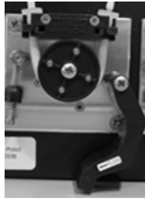
Pump Pressure Pad Unlocked
