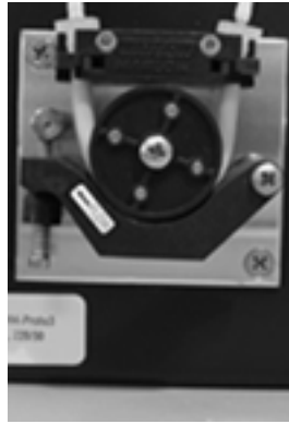
Pump Pressure Pad Locked
