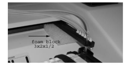
• Place the 3 x 2 x 1/2 foam block under the aspirate/dispense arm.
