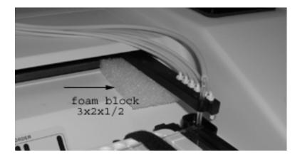
Close the aspirate shield, then tape the shield down to the instrument with write-on lab tape.
